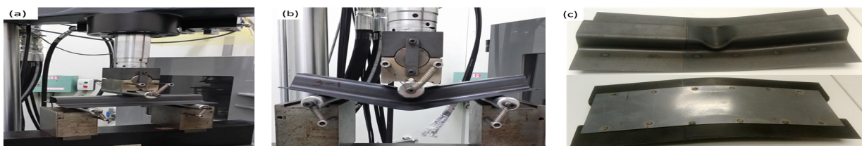
Fig.4. The apparatus and samples for the three-point bending test.
